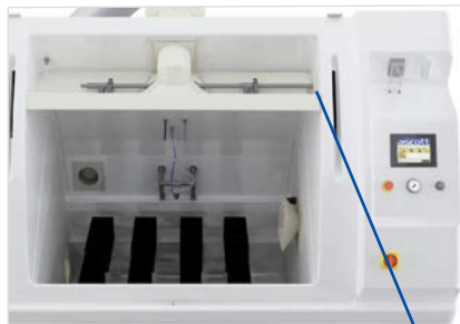
Magnetic drive disc on the end of the removable oscillating spray bar
