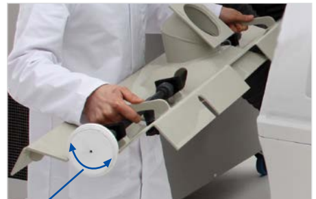
Magnetic drive disc on the end of the removable oscillating spray bar
